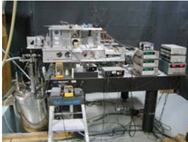
Figure 1. A 'quasi-optical' electron paramagnetic resonance (EPR) spectrometer.
