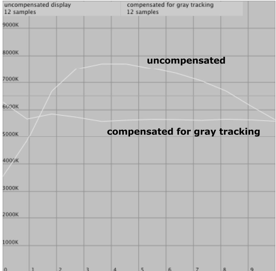
Figure 1. The correlated color temperatures of panels with and without gray tracking compensation. The target white point (set to 5700K) of the panel with compensation is much more stable across its dynamic range than that without.
