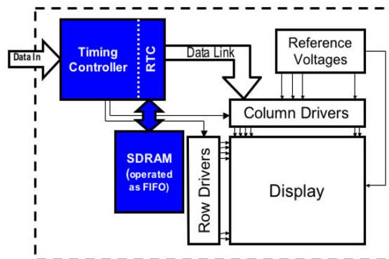
Figure 3. An example of RTC overdrive in the system. Highlighted is the added function of the timing controller in the LCD module. An external RAM is used as frame FIFO (first in, first out) memory.
