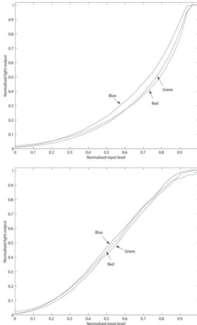
Figure 1. Output response of the primary colors as a function of the R, G, and B input levels for the LCD (top) and DLP projector (bottom).
