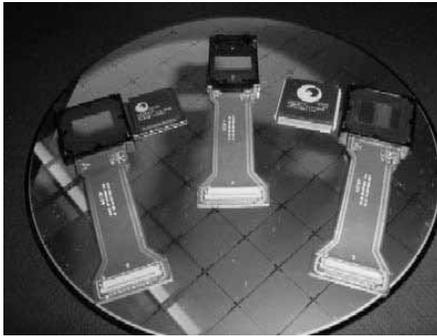
Figure 2. Aurora Systems liquid-crystal-on-silicon (LCoS) packaged imagers displayed on a backplane wafer.
