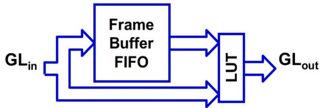
Figure 1. General block diagram of the RTC (response-time compensation) overdrive function.
