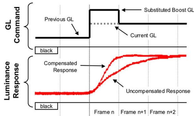
Figure 2. An example of RTC overdrive. A surrogate GL is substituted for the intended GL that causes the output to meet the intended luminance by the end of just one frame.
