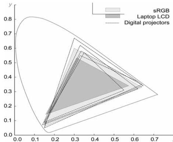
Figure 2. Chromaticity diagram comparing the gamuts of five different digital projectors to the sRGB display gamut and that of a typical laptop LCD display.
