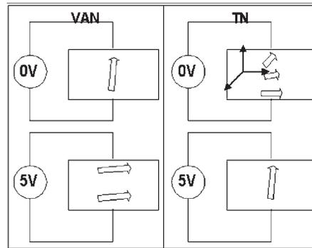
Figure 4. Representation of vertically-aligned nematic and twisted-nematic LC modes in the powered and unpowered states.
