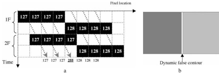
Figures 2(a) and 2(b). Example of a dynamic false contour.
