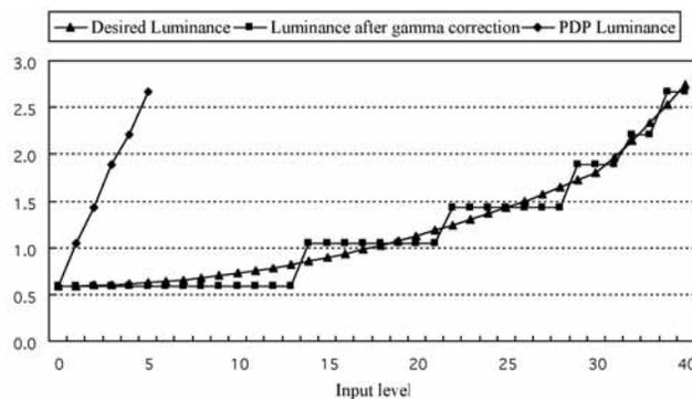
Figure 3. Example of inverse gamma correction.
