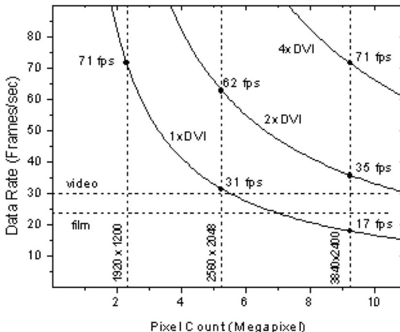
Figure 1. Data frame-rate limitations of DVI channels providing 165Mpixel/sec.
