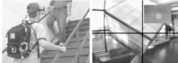
Figure 1. Left: RIT wearable eyetracker. Right: Video eyetracker record. The black crosshair indicates the observer's point of gaze in the scene.
