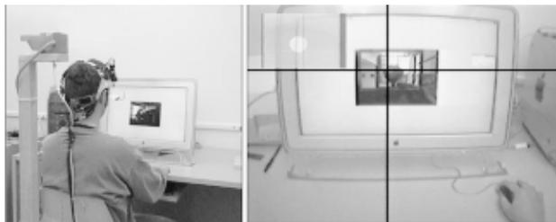
Figure 3. Left: observer wearing head-mounted eyetracker. Right: The black crosshair indicates the observer's point of gaze.
