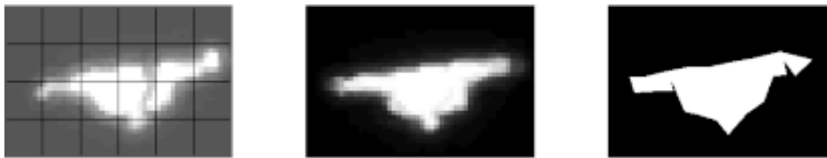
Figure 3. Left: example of partition into a set of subregions. Center: restored image, region-based approach. Right: restored image, edge-based approach.
