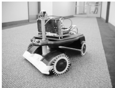
Figure 2. The low-cost Minnow robot platform (above). A simulation of the Minnow (right). →
