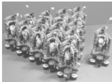
Figure 1. Two dimensional electro-magnetic unit system.
