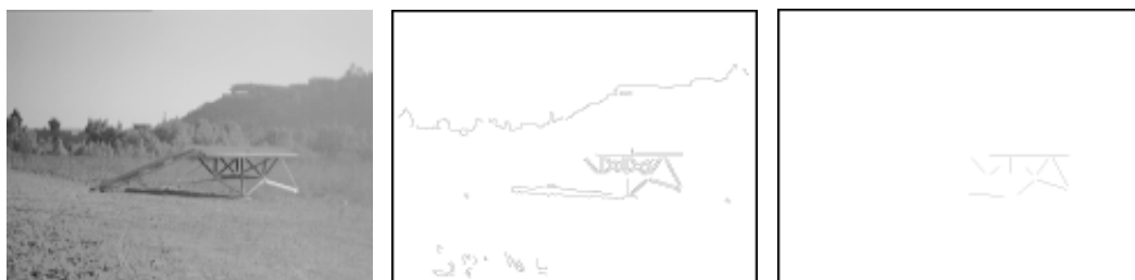
Figure 2. Truss structure features used for mid-range navigation. (Left) Original image. (Middle) Edge features. (Right) Truss structure features.
