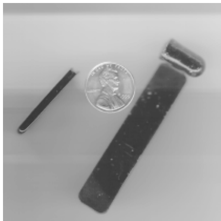
Figure 1. Photograph of thick photorefractive-polymer samples fabricated via injection molding.
