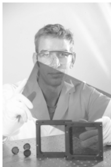
Figure 1. Three generations of BR-films. The earliest films had an aperture of \varnothing = 16\text{mm} in a \varnothing = 25.4\text{mm} mounting. The 90 \times 90\text{mm} large-aperture films come in a 4" mounting and have an active area about 40x bigger than the conventional BR-films. The BR-D96N film (left) is completely bleached, whereas the BR-WT film (right) is in its initial purple state. The 8 \times 12\text{in} BR-film in the rear is a prototype.
