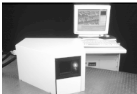
Figure 2. The FringeMaker™ system for non-destructive testing and vibration analysis uses 4" size BR-films for recording.
